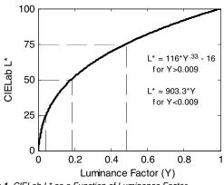
Figure 1. CIELab L\* as a Function of Luminance Factor
