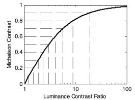
Figure 3. Michelson Contrast as a Function of Luminance Contrast Ratio
